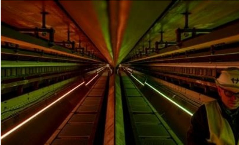
A split in the hyperloop tube allows vehicles to change directions
