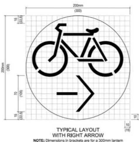
Figure 2: Dimensions for typical directional cycle signal lantern aspect layout
