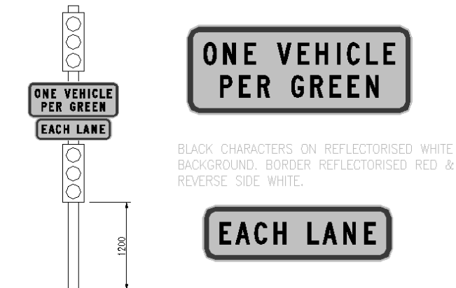
Figure 3: Ramp Meter Display A
