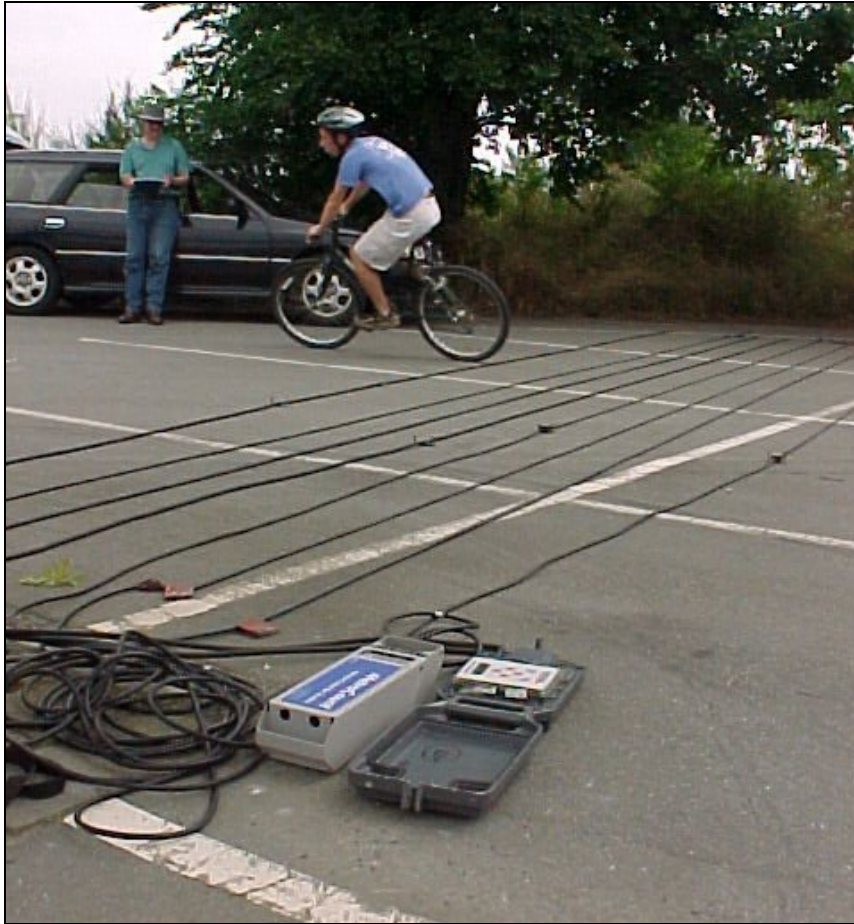
Figure 3: MC 5600 (left) and GR M410 (with case open) counters tested in a carpark, free of other traffic, using four different kinds of pneumatic rubber tubes
