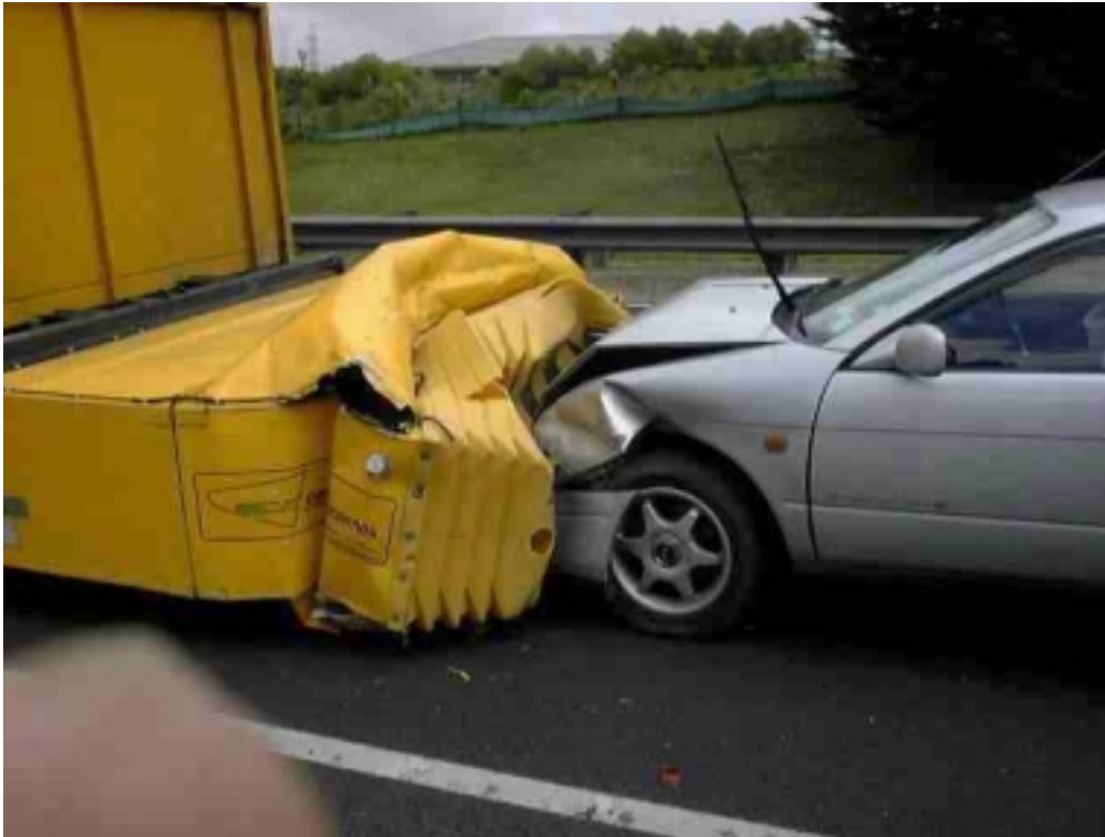
Figure 2 Result of impact of car with truck-mounted attenuator
