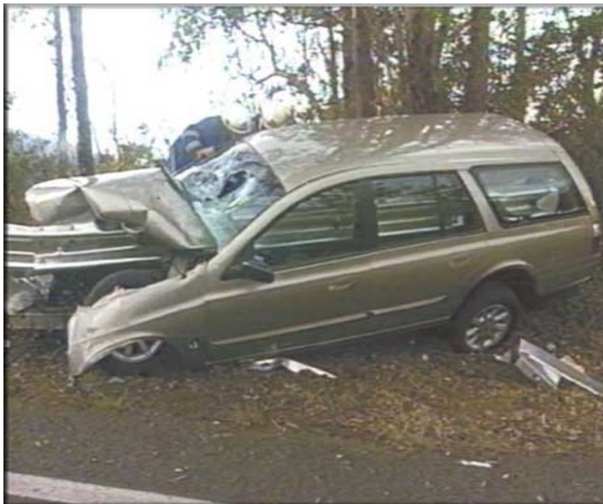
Figure 1 Result of impact with guardrail terminal,
