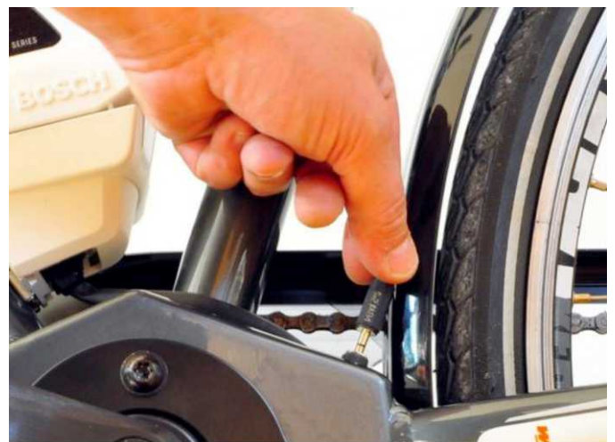
Figure 4: Installing a dongle renders the control panel readout inaccurate but doubles the speed limitation from 25 km/h to 50 km/h (although most EU standard 250 watt motors are not powerful enough to propel an e-bike beyond 40 km/h) image source: pro-cycling.golla.com
