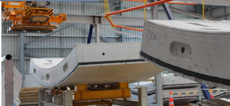
Some of the 12,000 precast concrete ring segments produced so far.
