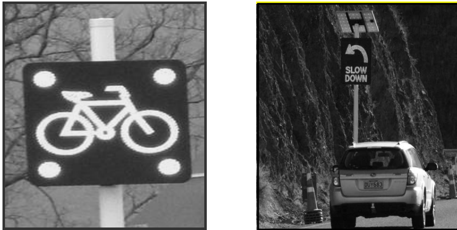
Figure 1: Cycle activated cyclist warning sign (left), vehicle activated curve warning sign (right).
